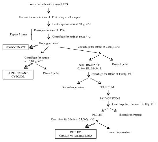
**Fig. 2** Schematic representation of the mitochondrial isolation steps for the PK assay protocol. *C* cytosol; *H* homogenate; *ER* endoplasmic reticulum; *L* lysosomes; *MAMs* mitochondria-associated membranes; *Mc* crude mitochondria; *Mp* pure mitochondria; *PK* proteinase K
