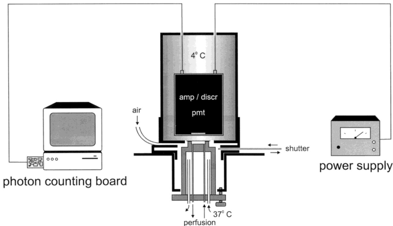
Fig. 6. The aequorin measuring system. pmt=photomultiplier; amp/discr = amplifier/discriminator. The photomultiplier is kept in a cooled dark box, the cell chamber at room temperature. During manipulations on the cell chamber, the photomultiplier is protected from light by a shutter. During aequorin measurements, the shutter is
